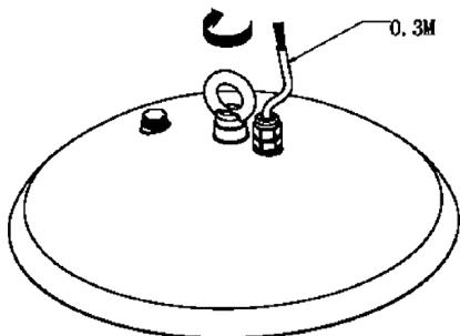
2. To change the wattage settings, loosen the sealing cap using a spanner. Skip this step if you prefer to use the default output.
