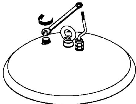
5. Hang the luminaire by the suspension ring, attaching it to a fixed safety hook or closed link chain.
