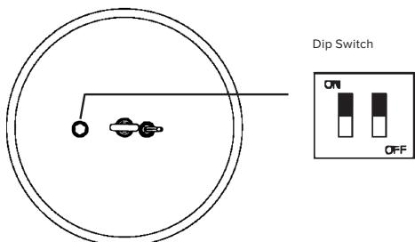
3. Adjust the lighting level to your desired lumen output using the lumen select switches. If you're using the default output, disregard this step.
